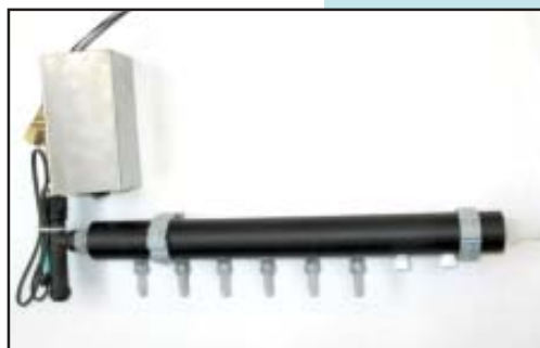
Beta's new approach to flush manifold check valves reduces clogging and trouble calls. The integral flow switch and pressure switch stop the chemical pumps if flush water is unavailable or if pressure builds up in the manifold. Never get sprayed with chemicals again!
