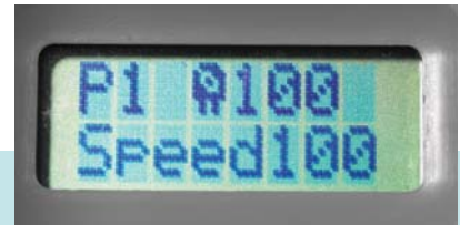
Summit E Pump Speed Control Screen
