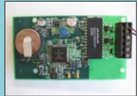
The heart of Summit's datalogging and reporting capability is the Data PCB.
