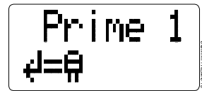
Screen 3. Prime Pumps
