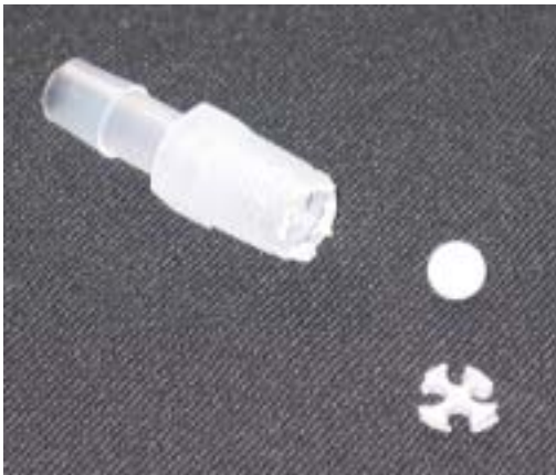
Old Check Valve Assembly
